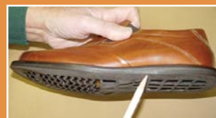
Sand to proper thickness
