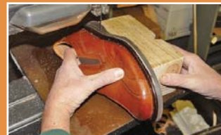
Removing most of sole with band saw or sharp knife
